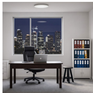
With insufficient ambient light, the sensor turns on the light and dim to 100% brightness when human motion is detected.
